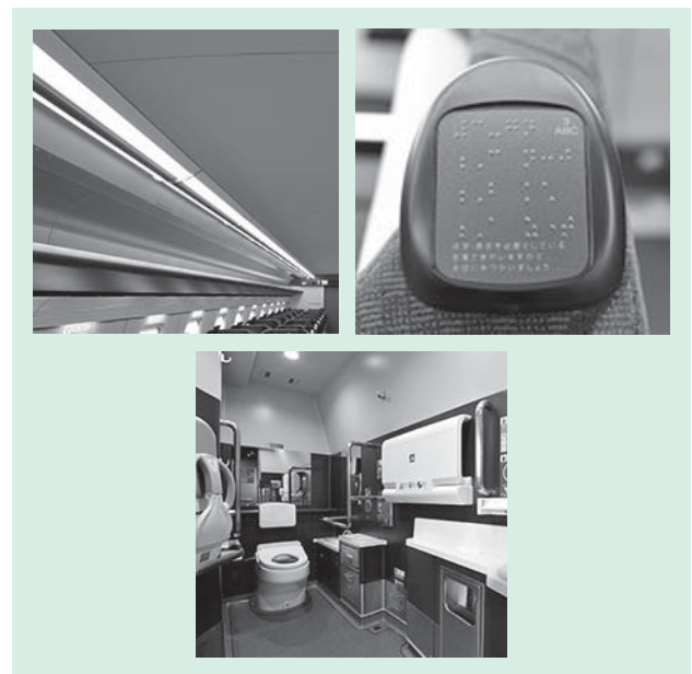
Fig. 3—Interior Fittings on Latest High-speed Shinkansen Rolling Stock. The internal fittings use the latest technologies such as LED lighting and are designed for barrier-free accessibility.
