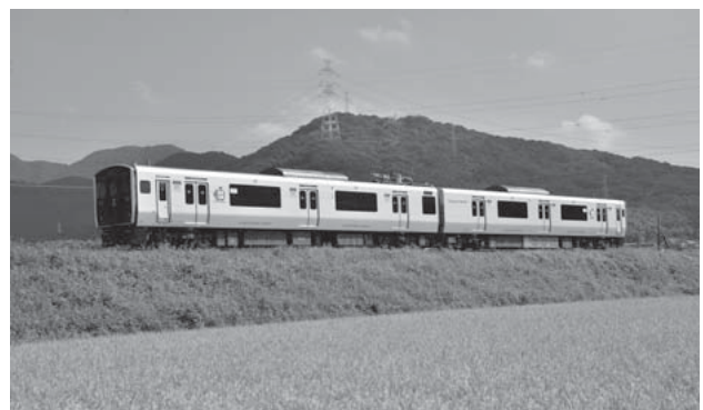
Fig. 3—Prototype Battery-powered Train. The 83 kWh of high-capacity lithium-ion batteries installed under the floor store energy when traveling on electrified sections of track and provide the energy to run on non-electrified sections.
