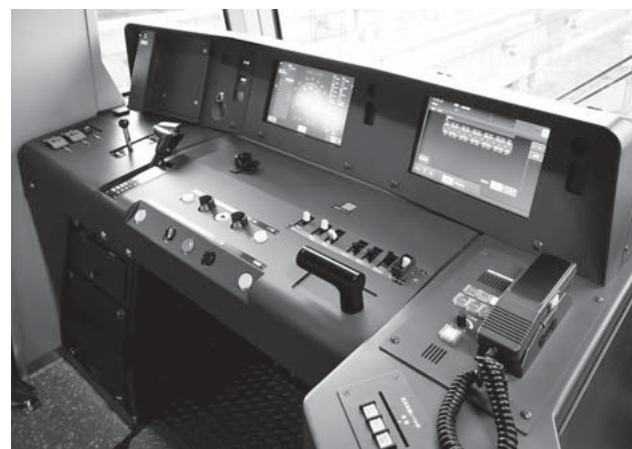
Fig. 11—Control Panel for Tokyo Monorail Series 10000. The control panel has two monitors. A pop-up display format is used to improve operation.
