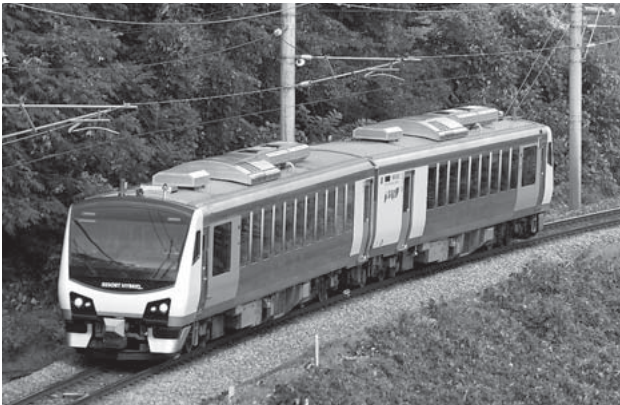
Fig. 1—Series HB-E300 Resort Train. Lithium-ion batteries that can provide 15.2 kWh are installed on top of each car.
