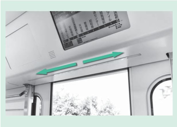
Fig. 5—Indicator Lights for Opening and Closing Doors. The indicator uses two-color LEDs (red and blue) to display a repeating pattern of moving lights in which elements progressively turn off in the directions shown by the arrows.
