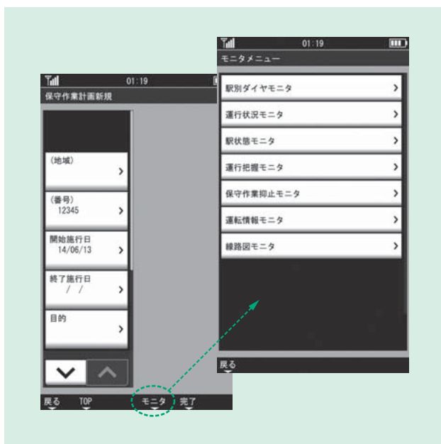
Fig. 5—Shortcut for Calling Up Monitoring Functions. Shortcut keys have been assigned to almost all screens to facilitate switching to monitor function screens.
