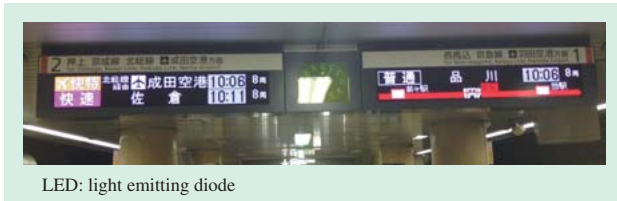
Fig. 5—Full-color LED Passenger Information Display for Asakusa Line.
