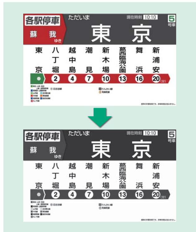
Fig. 6—Consideration for Elderly People and People with Color-impaired Vision. Color displays are checked in black and white, and adjusted to use colors in ways that are easy for the elderly people and people with color-impaired vision to distinguish.
