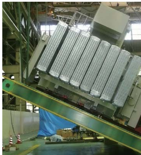
Inclination test of transformer. Because the transformer will be installed on a floating platform, it needs adequate measures for dealing with swaying.
