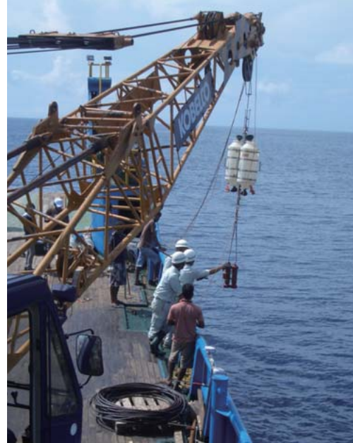
A bathymetric survey is being conducted in the Maldives in preparation for the use of deep seawater.
