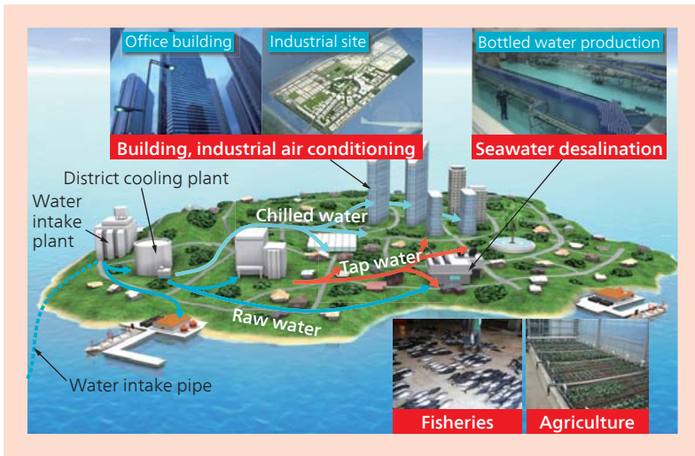
A plan is underway in the Maldives to use deep seawater first to produce chilled water for air conditioning, and then for a series of other uses.
