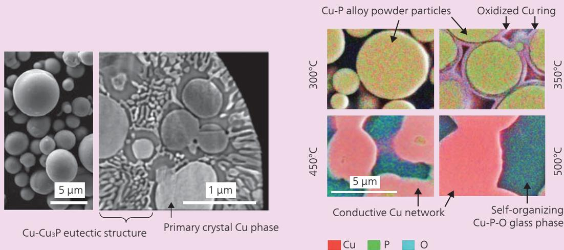
Note: The illustration of the atmospheric sintering process was created by compositing a chemical composition map obtained from energy dispersive X-ray analysis on an SEM photograph of an application film cross-section.
