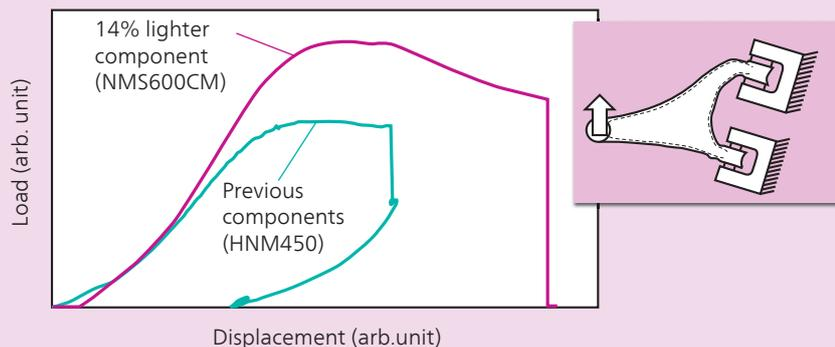
5 Example applications for NMS600CM in lightweight suspension arms (top) and the load-displacement graph obtained by bench testing an upper arm for passenger cars (comparison of previous Hitachi model and lightweight NMS600CM) (bottom)
