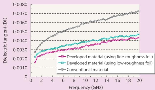
6 Transmission loss measurement result for developed material (top) and electrical characteristics (frequency dependence of dielectric constant/dielectric tangent) measurement result (bottom)
