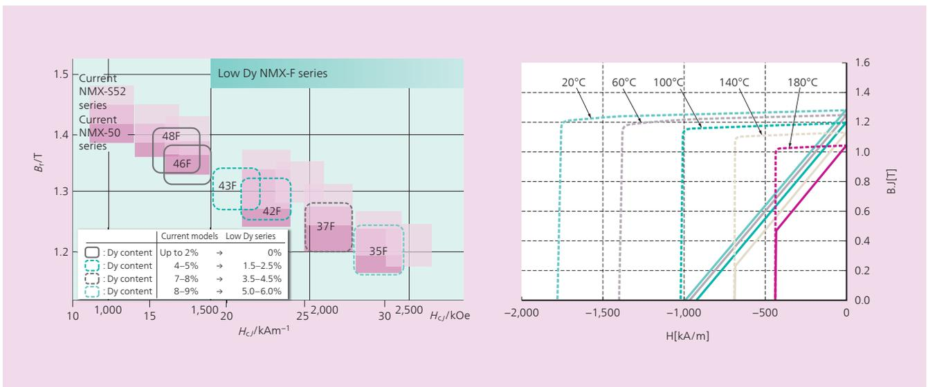
3 Low Dy magnet lineup (left) and temperature characteristic curve of NMX-42F (right)
