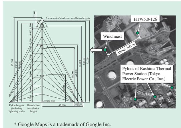
Fig. 2—Aerial Photograph of the HTW5.0-126 Prototype Turbine Site and Side View of the Wind Mast.
