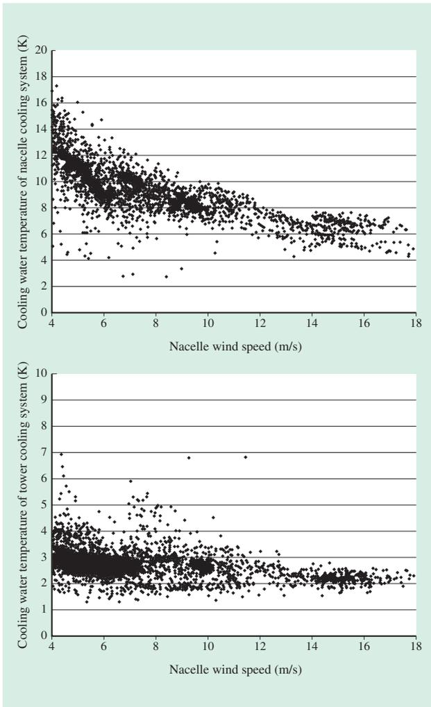
Fig. 6—Correlation between Cooling Water Temperature and Nacelle Wind Speed.
