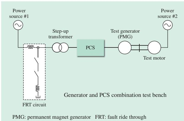
Fig. 4—Factory Testing Configuration (FRT Function Verification).
