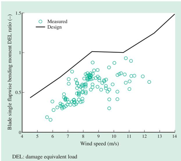
Fig. 8—Flapwise Bending Moment Fatigue Load at Blade Roots. The graph shows 10 minutes of fatigue equivalent load values for blade flap bend relative to the average wind speed over a 10-minute period.
