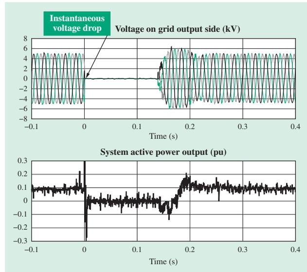
Fig. 5—Example FRT Function Test Waveforms.
