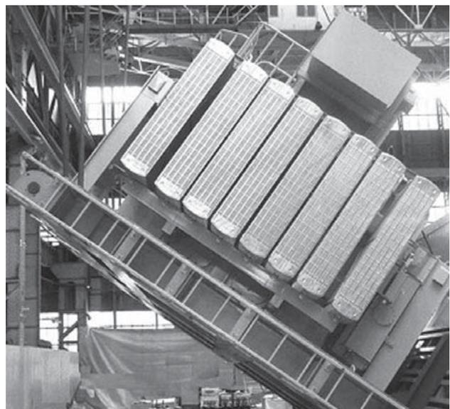
Fig. 10—Transformer Tilt Test. The photo shows the transformer tilt test done at a test facility in Kokubu Works of Hitachi, Ltd.
