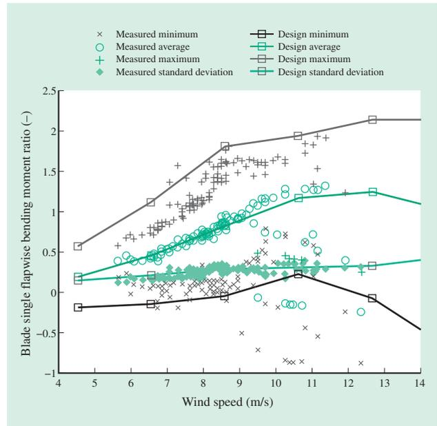
Fig. 7—Statistical Values of Flapwise Bending Moment at Blade Roots.
