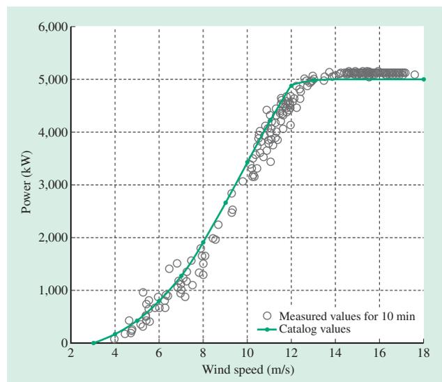
Fig. 3—Measured Power Curve Values. The curve shows the correlation between the power and the wind speed measured by the wind mast at the height of the wind turbine hub. The performance obtained closely resembles the anticipated catalog values.
