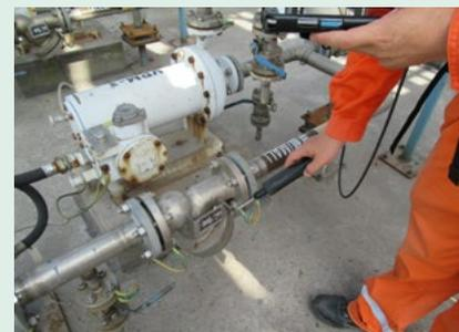
Detecting a VOC leak.
